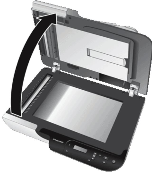
3. Clean the white strip on the inside of the scanner cover and the clear scanning strip on the scanner bed. Wipe these items with a clean, damp, lint-free cloth.
