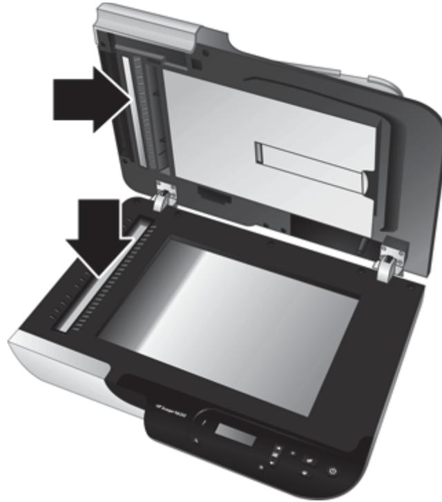
4. Open the ADF access door (1) and the roller cover (2) inside the ADF.
