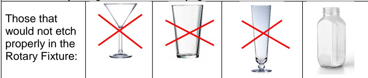
Glassware with flat vertical sides can be etched if they are not taller than 4 inches when laid on their sides:
