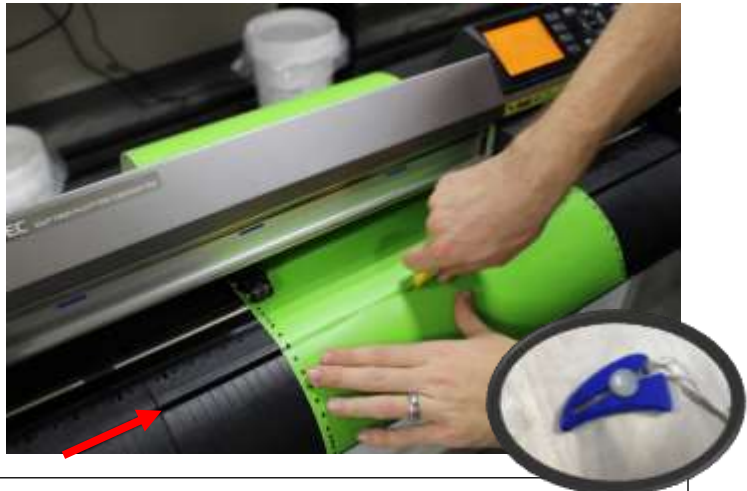
Figure 19 – Cut off the Vinyl above the design work by pulling your Cut-off Knife through the Cut-off Groove
