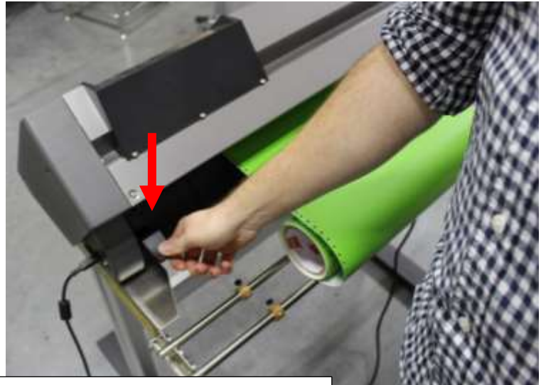
Figure 1 – Lowering the Media Set Lever Shown on the Backside of the Machine
