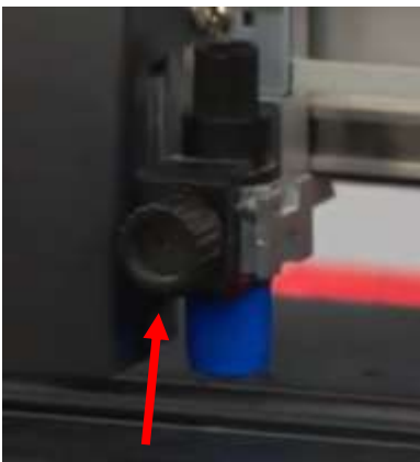
Loosen the "Tool Holder Screw/Knob" by turning it counter clockwise
