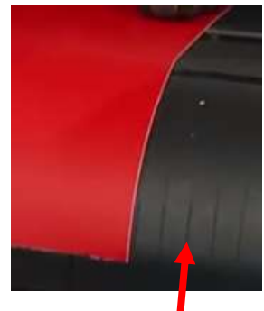
Figure 4 – Parallel raised lines to help you make sure the vinyl is coming in straight
