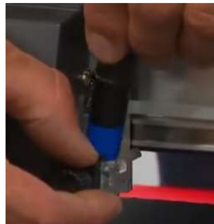
Lift the tool up and out, being careful NOT to touch the blade protruding from the blue end
