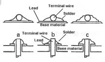
c) Bad soldering of terminal wire and PCB trace. This is a "cold" solder joint where the soldering iron was not held on the joint long enough to heat the joint sufficiently and where some movement of the joint could have occurred before the solder cooled. It will appear to have a rough textured surface. This can be corrected by reheating the joint until the solder flows and adding a small amount of flux.
