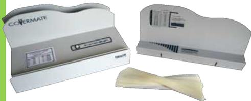
The System has a binding repair machine that fixes a variety of types and sizes of books. This machine easily binds up to a 2½" thick book and it has a sliding wall to hold smaller books in place. It will also work with legal size as well as regular 8½ x 11" size items. Repaired books will be ready to use in just 20 minutes! Go to <http://www.coverone.net> and click on the link for Book Repair Demo on the left-hand side of the page to see it in action.
